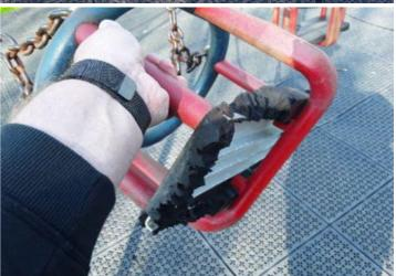
**Finding:** The seat is severely damaged and requires replacing
