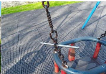
**Finding:** The connecting links are in excess of 8.6mm and less than 12mm and fail the requirements of BS EN 1176
