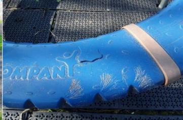
Finding: The casing is cracked in a number of places and rough edges are exposed in two areas
